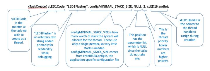
Figure 5 - Explanation of parameters passed to the xTaskCreate routine.
