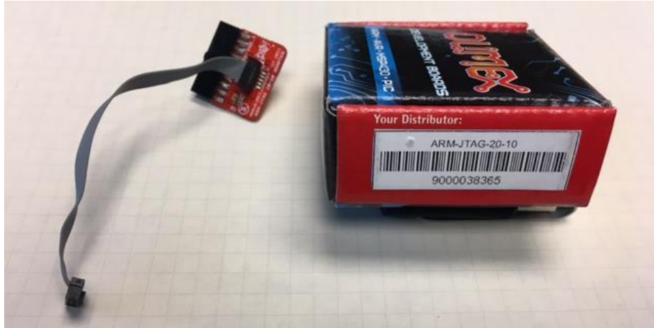
Figure 2 - Olimex harness for connecting to standard 0.05" x 2 row JTAG interface
