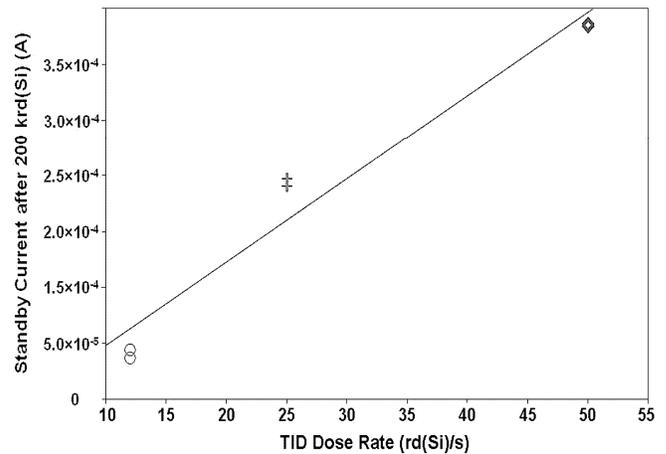
Fig. 5. Standby current after 200 krd(Si) vs. TID dose rate for the hardened parts. The increase in current post radiation decreases linearly with the dose rate, suggesting little or no change at the dose rates in most orbits.
