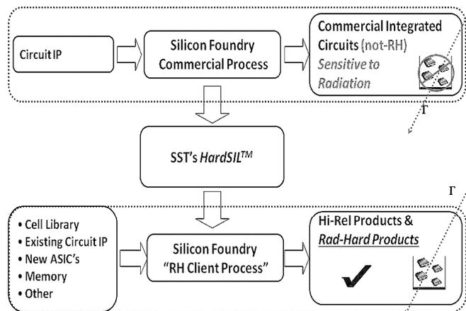
Fig. 1. SST manufacturing model at a commercial foundry with HardSIL™ process enhancements added to create a radiation-hardened silicon process – the “RH Client Process.”
