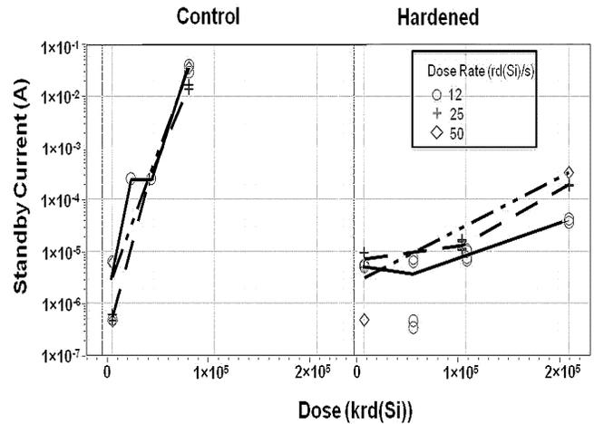
Fig. 4. Standby current vs. TID as a function of dose rate for control and hardened samples. The standby current for the hardened samples decrease with dose rate. The current is unaffected by the dose rate for the control samples.
