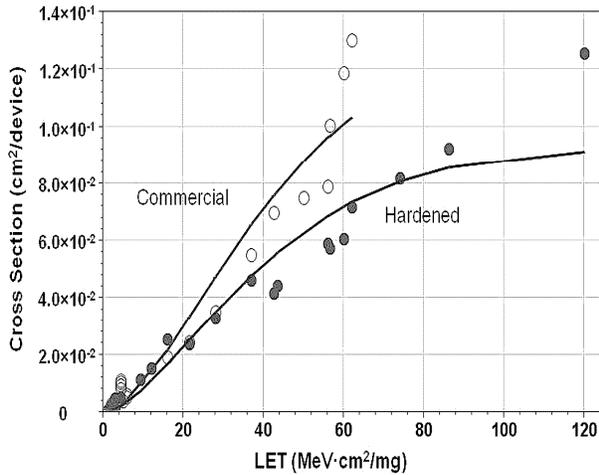
Fig. 7. Device cross sections and Weibull fits as a function of effective LET for the VC33 DSP memory. While the onset for both samples is similar, the saturation cross section is lower for the hardened device. The cross section for both parts deviated significantly from the Weibull fit at high LET's.
