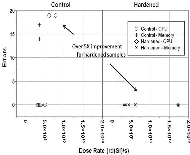
Fig. 6. Dose rate testing results showing no errors for the hardened part at the maximum achievable dose rate.
