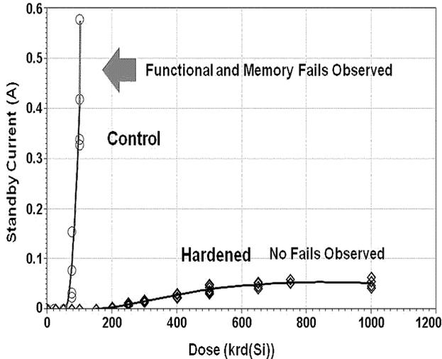
Fig. 3. Standby current as a function of total dose for the hardened and the control samples. The hardened sample showed no functional failures after 1 Mrd(Si) where the control sample failed after less than 100 krd(Si).
